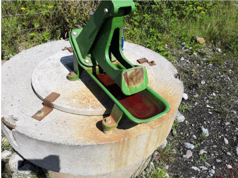
Plate 2 – Example Cattle nose pump on groundwater well
